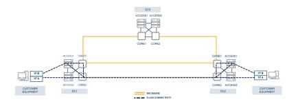
**E-Lan:** Designed to connect multipoint to multipoint across the entire network and configured as a single unprotected linear circuit or deterministic protected connection.
